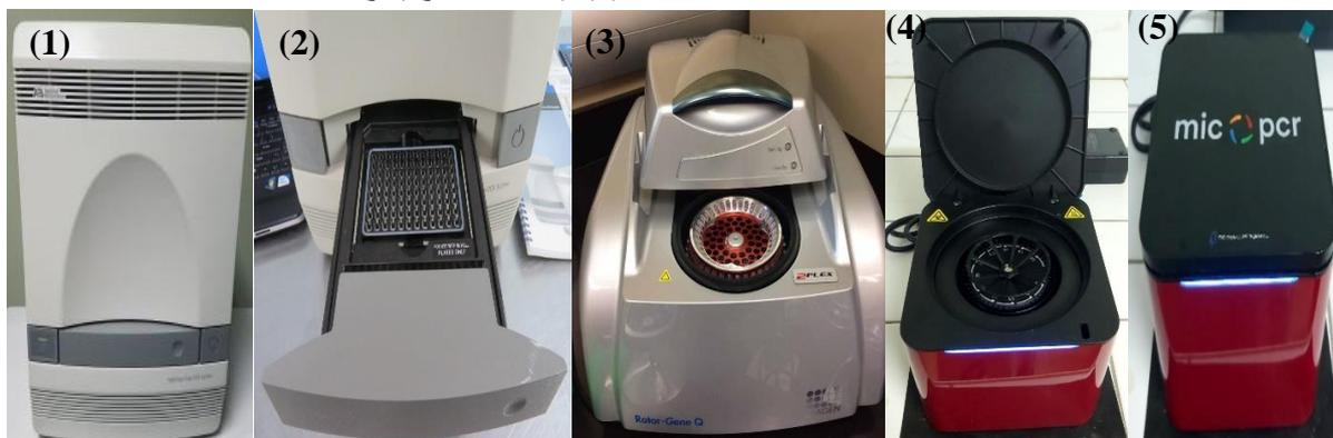
Figure 34: Automates d'amplification (thermocycleurs).
